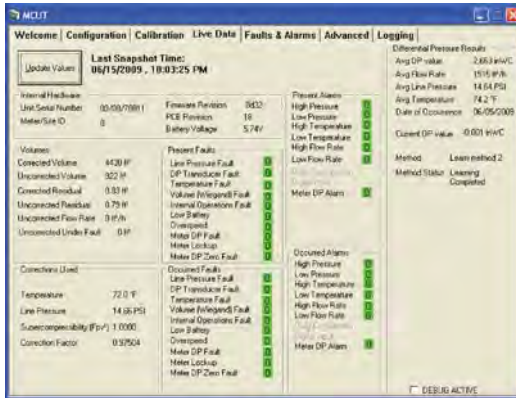
Live data screen displays current DP read, as well as last valid DP read, pressure, temperature and flow rate with date of occurrence.
